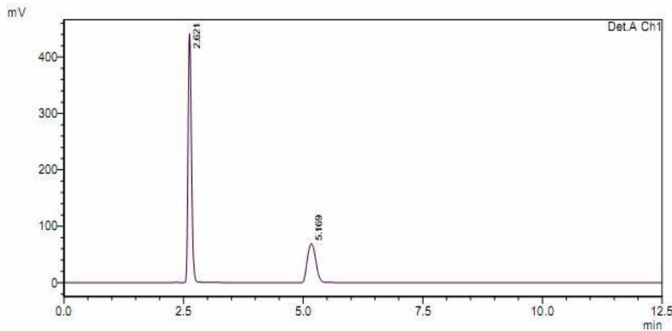
**Result:** The retention time of Atenolol was 2.621 min and for Nitrendipine was 5.169 min. The peaks are well separated with a resolution of 11.079.
