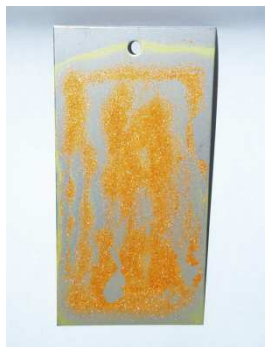
SS coupons are spiked with sample soil (s).
