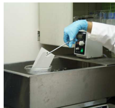
Coupons are exposed to multiple cleaning parameters depending upon customer's objectives.
