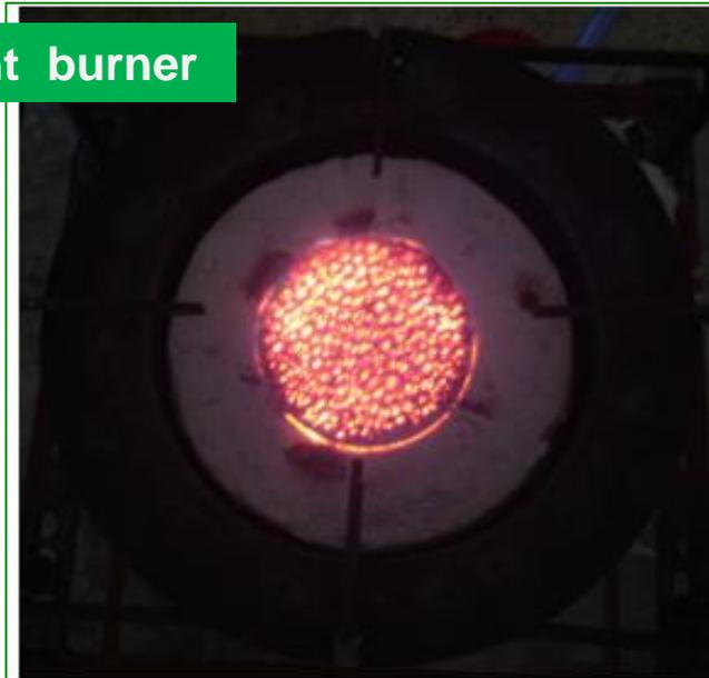
$$\eta_{th} = \frac{(m_w C_{pw} + m_v C_{pv})(T_2 - T_1)}{m_f \cdot CV} \times 100$$
