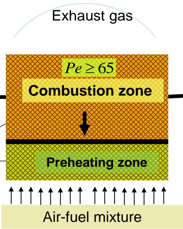
Heat transport for reaction zone stabilization
