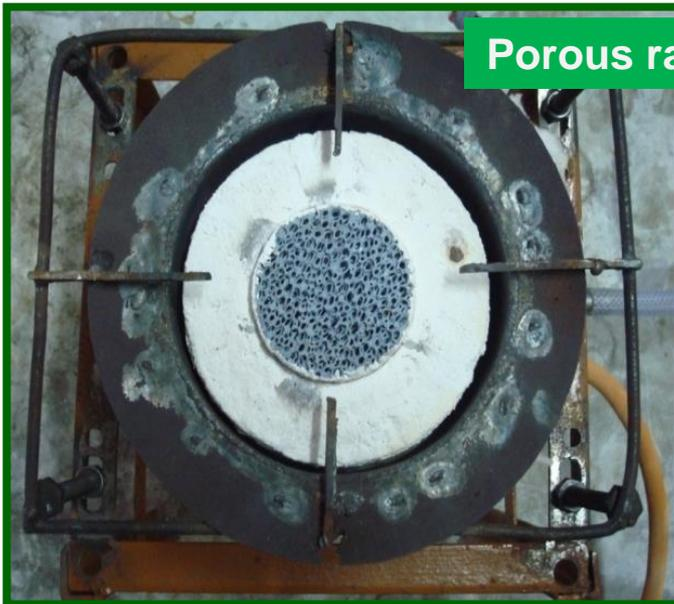
Porous radiant burner
