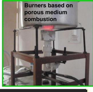
Combustion in porous media is efficient
