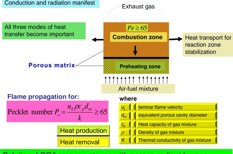
Solution: LPG/kerosene stoves with porous radiant burner
